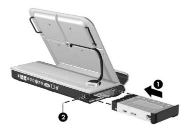
Installing the Hard Drive Carrier
